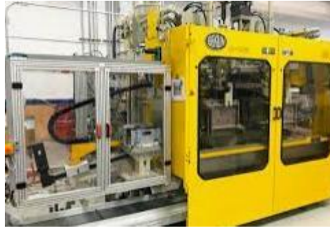
Gambar 3.6 Injection blow molding
