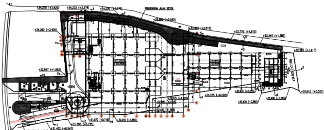
Gambar 3.7 Denah Dinding Penahan Tanah Gereja SPMBG
