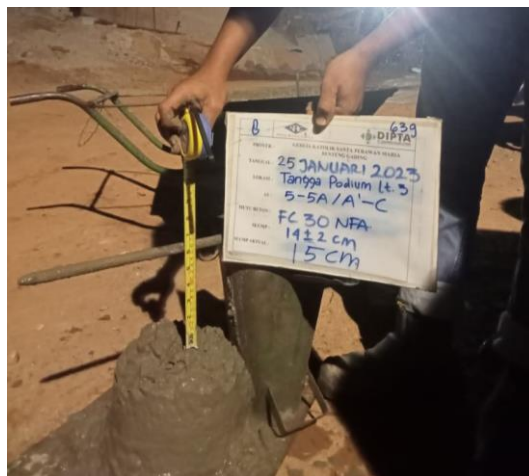
Gambar 4.1 Slump Test
