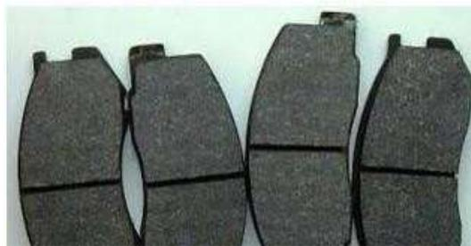
**Gambar 2. 5** Kampas Rem Berbahan Baku Non-Asbestos
