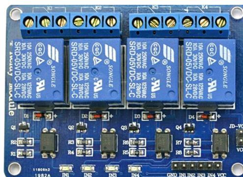
Gambar 2.3 Relay Module 4 Channel Arduino
