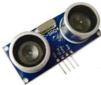
Gambar 2.7 Sensor Ultrasonik [29]
