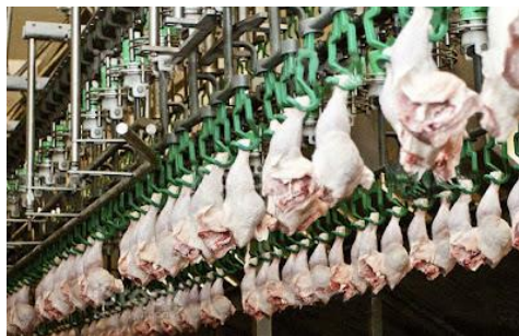
Gambar 2.3 Proses Pencabutan Bulu ( Defeathering )
