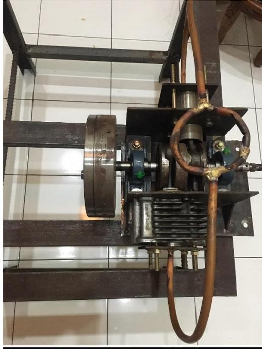
**Gambar 4.1** Prototipe Mesin Stirling
