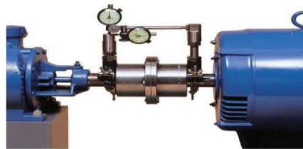
Gambar 3.8 Metode Alignment Dial Indikator
