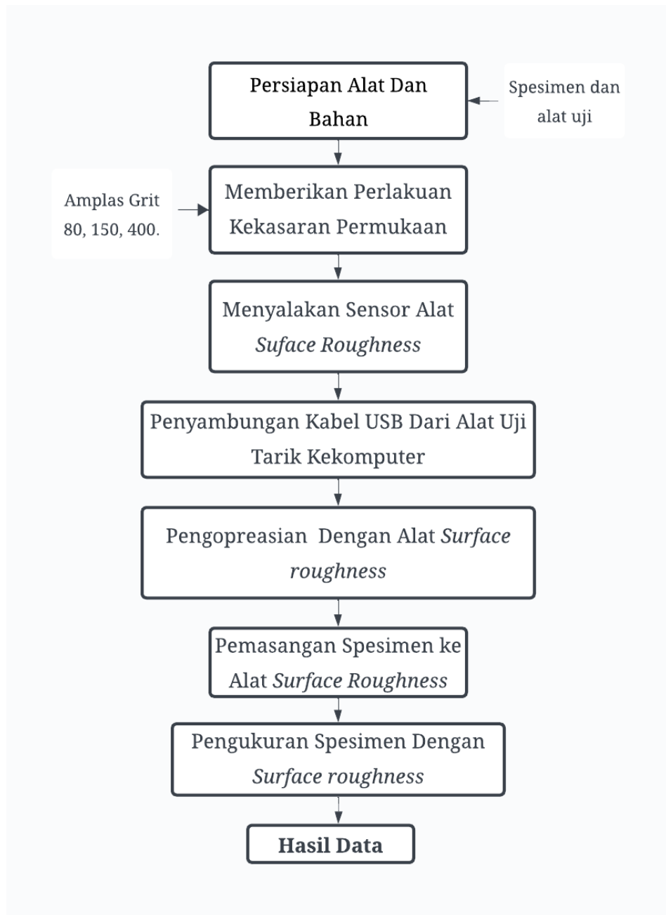
Gambar 3.8 Proses Pengukuran Surface Roughness
