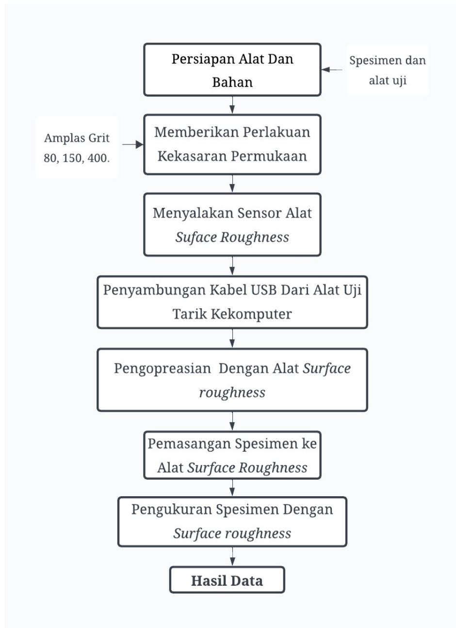
Gambar 3.8 Proses Pengukuran Surface Roughness
