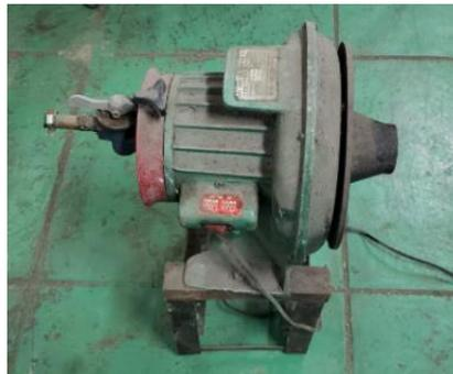
**Gambar 2. 6** *Rotary Cup Oil Burner*
