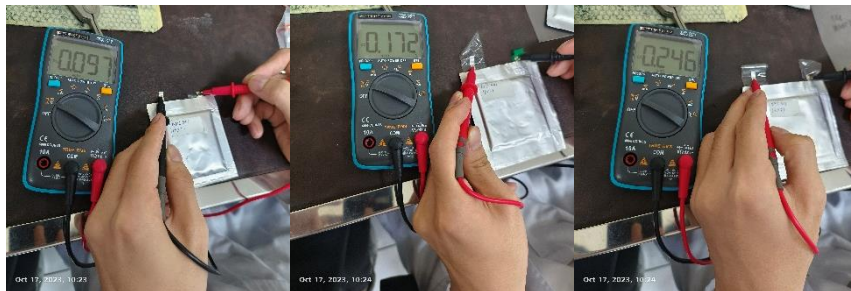
Gambar A.6 Pengecekan Voltase awal (0 V Jika Short )
