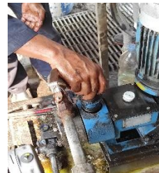
Gambar 4.13 Melepaskan Hydraulic Filter Oil
