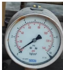
Gambar 4.3 Kondisi Discharge Pressure awal Injection Pump
