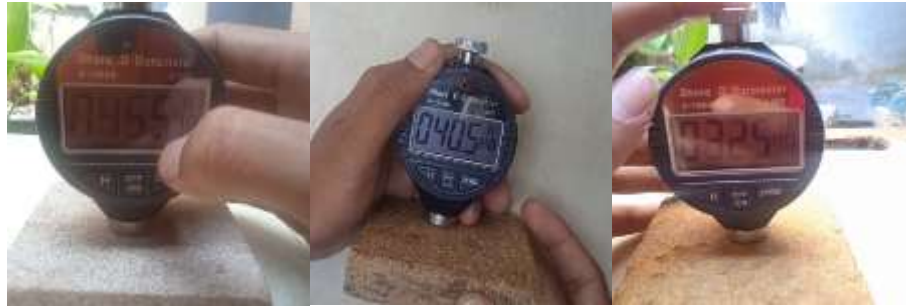
Gambar C.9 Proses Pengujian Kekerasan Shore D
