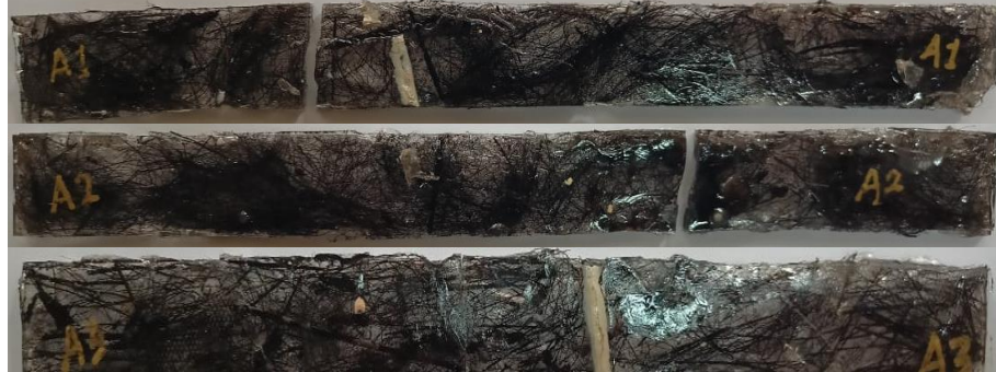
Gambar B.1 Sampel Uji Tarik A
