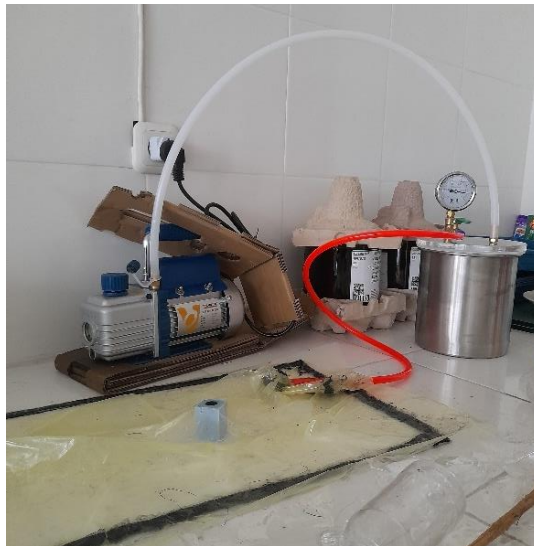
Gambar 4.2 Hasil Rancangan Alat Vacuum Bag
