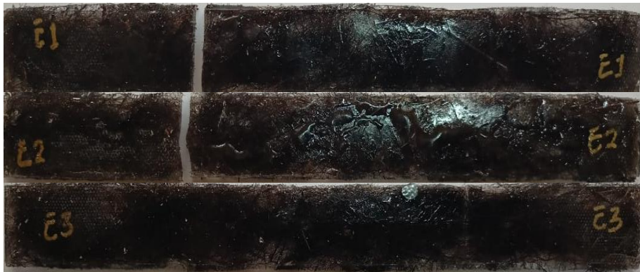
Gambar B.5 Sampel Uji Tarik E
