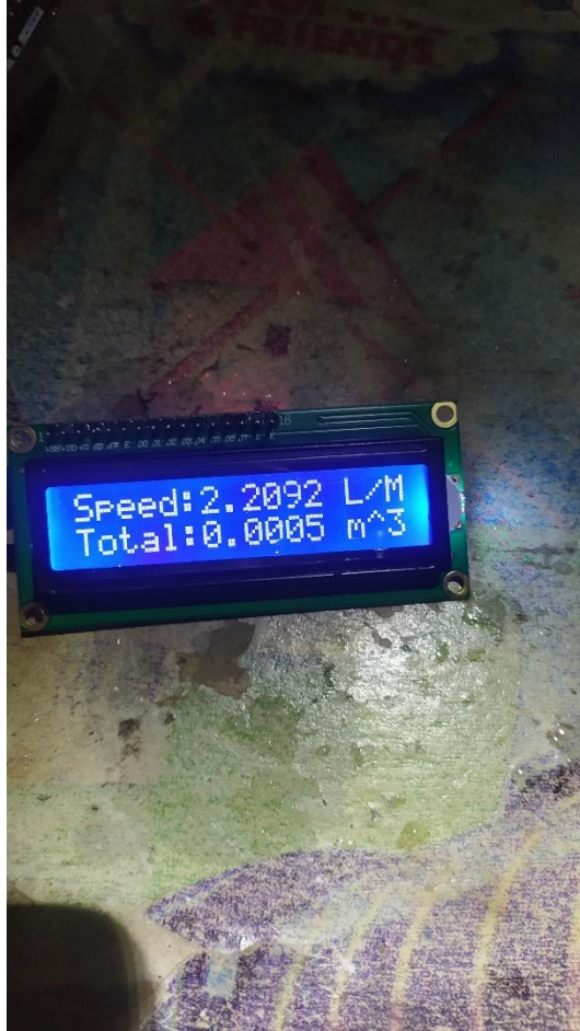
Gambar 1 Tampilan LCD Kalibrasi Flowsensor
