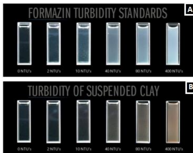
Gambar 2.2 Formazin Turbidity Standards , (A) Turbidity of Suspended Clay , (B) Sampel Kualitas Air [17]
