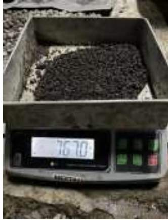
Gambar 5.7 Pengujian Kadar Lumpur Agregat Halus (Sumber: Qurrotul Milania, 2023)
