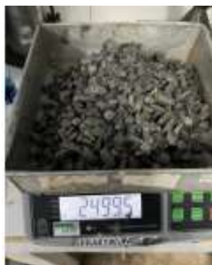
Gambar 5.4 Pengujian Kadar Lumpur Agregat Kasar (Sumber: Qurrotul Milania, 2023)
