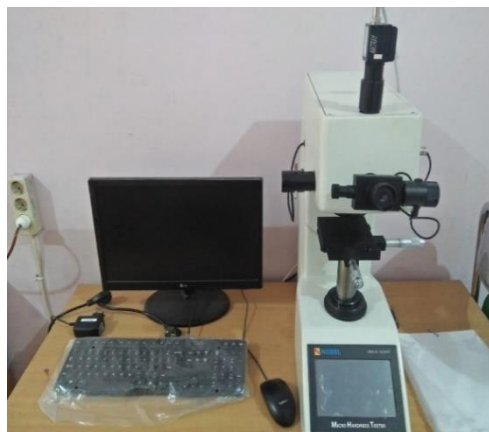
Gambar 3.10 Alat Uji Micro Hardness Vickers
