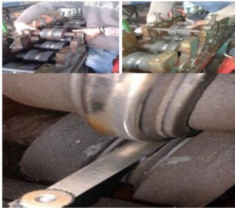
Figure 6 Measurement of Roll Gap
