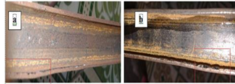
(a). Wings are not Perfectly Bent. (b). Material Damage.
