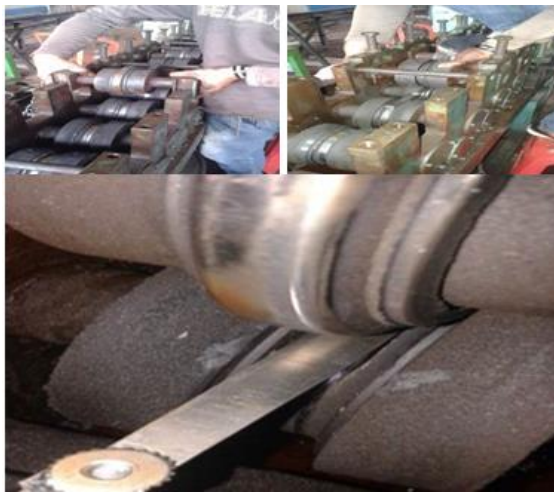
Figure 6 Measurement of Roll Gap
