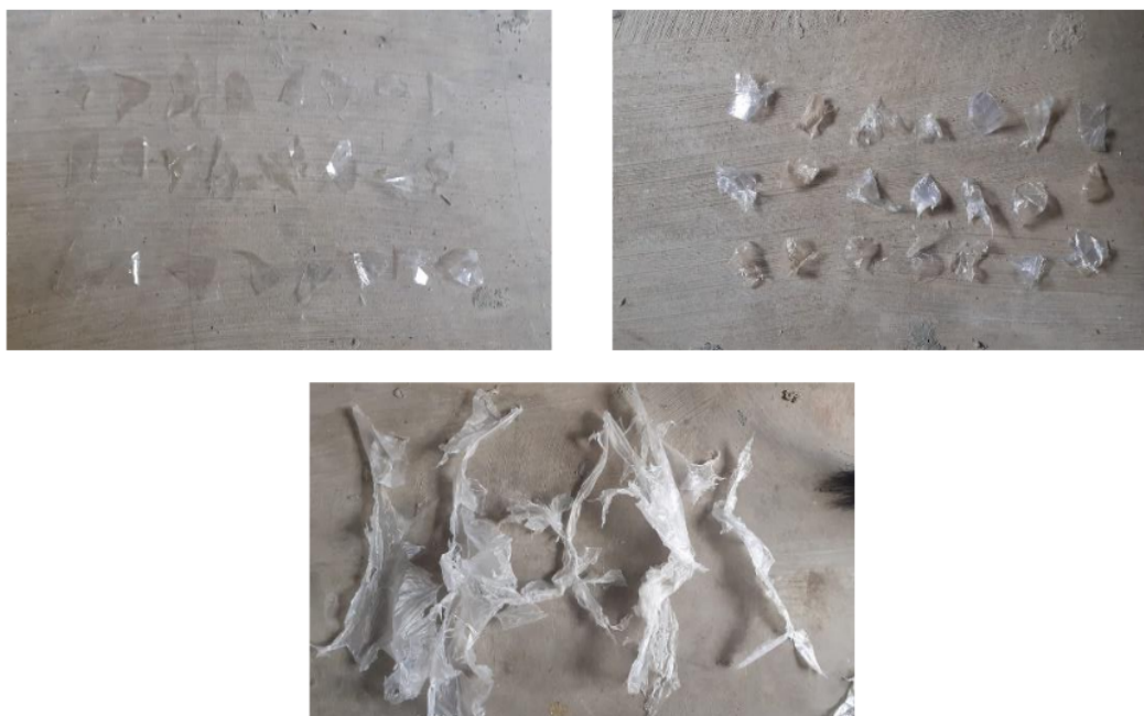
Figure 4. Size of plastic waste after cutting by shredder machine plastic
