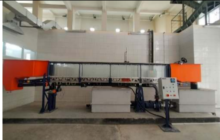
Gambar L-4.1. 1 Glass Sided Tilting Flume (Armfield S6-MKIII)
