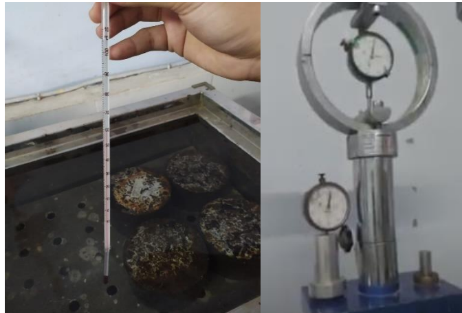
Gambar 5.23 Pengujian Marshall Sisa
