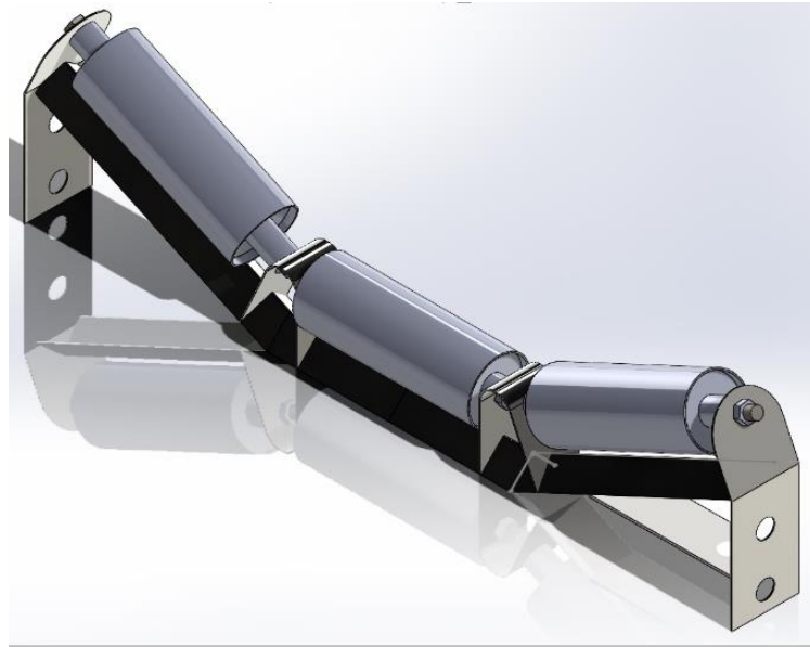
Gambar 4.8 Carrying Idler 1/Troughed Idler 1
