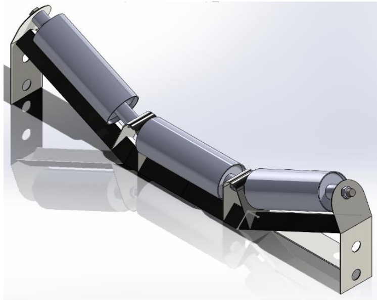
Gambar 4.20 Carrying Idler 1/Troughed Roller 1
