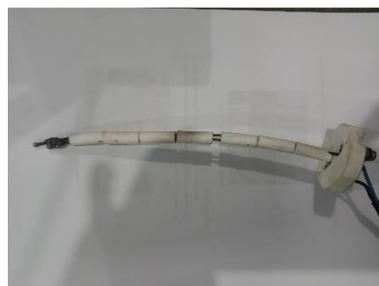
**Gambar 3.4** Thermocouple K
