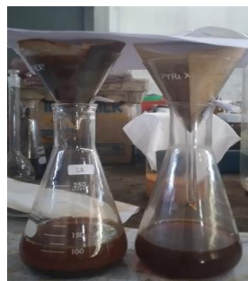
Gambar 3.4 Proses Filtrasi Larutan Hasil Pelindian
