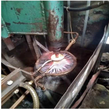
Gambar C.1 Induction Electromagnetic Furnace
