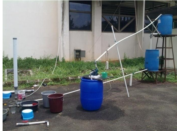
Gambar 3. Sistem instalasi model pengujian hydraulic ram pump .
