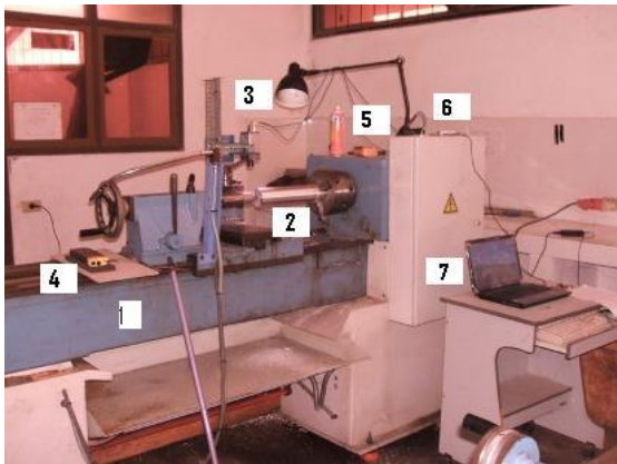
Gambar 1 Set-up peralatan eksperimen pemesinan magnesium (1) mesin bubut, (2) magnesium, (3) kamera CCD-IR, (4) termometer dijital, (5) termometer dijital, (6) video adapter, (7) notebook
