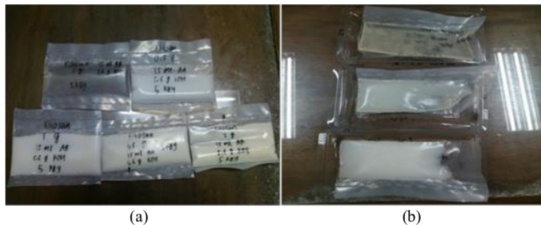
Figure 1. Superabsorbent hydrogel (a) variation of chitosan (b) variation of gamma irradiation dose with 0,5 g of chitosan
