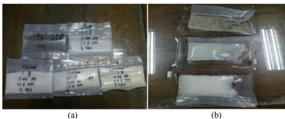
Figure 1. Superabsorbent hydrogel (a) variation of chitosan (b) variation of gamma irradiation dose with 0,5 g of chitosan
