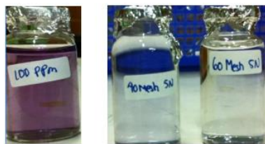
Gambar 4. Sampel larutan methyl violet; a. Sampel awal; b. Sampel setelah proses adsorpsi
