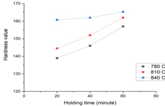
**Figure 4.1 Chart between hardness value and holding time**
