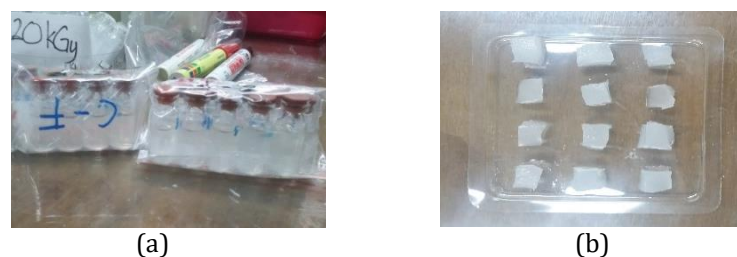
Figure 1 Change in the material's shape during the preparation: (a) Before irradiation; (b) Hydrogels of (pNIPAAm-chitosan-PVA) that have been cut after irradiation
