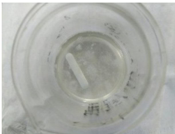
Fig. 10. Flocculation during the mixing at high level of chitosan.
