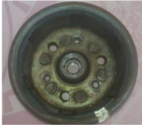
Gambar 2 Magnet Rotor
