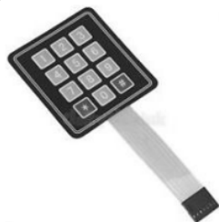
Gambar 4. Keypad matrik 4x3
