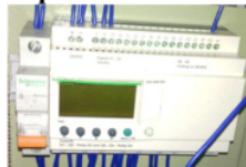
Figure 2. PLC (Smart Relay Zelio) [8]
