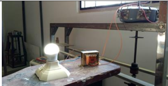
Fig 5. Generator AC with Translation and Rotation Mechanism by using load LHE 5 w.
