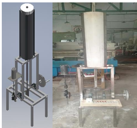
Figure 1. Design of generator translation and rotation motion in vertical direction
