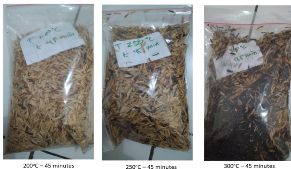
FIGURE 2. Color changes in the torrefaction of the torrefaction process with temperatures of 200, 250 and 300°C and 45 minutes holding time.
