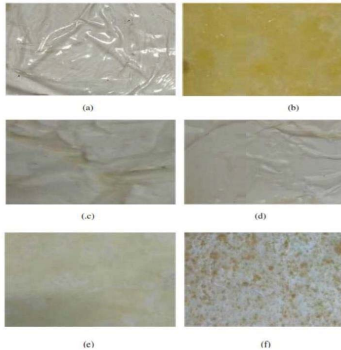
FIGURE 1. Visual form of blend film with OLLA/starch ratio (a) 0/100; (b) 100/0; (c) 20/80; (d) 40/60; (e) 60/40; (f) 80/20
