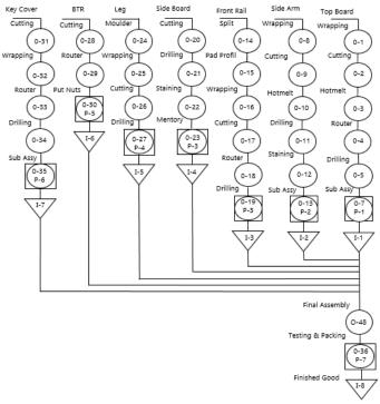
Fig. 2. Operation process chart of side board
