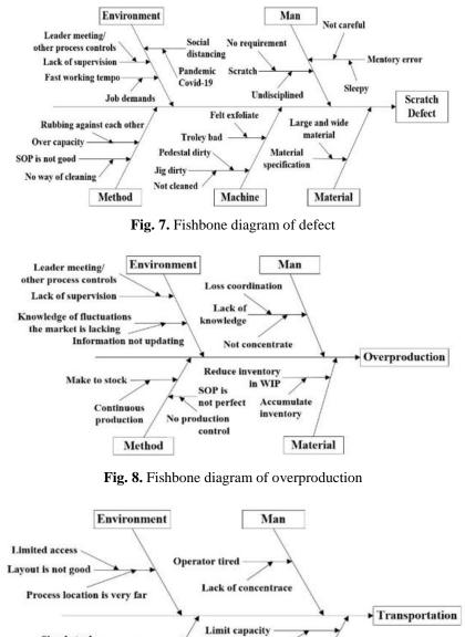
following analysis of the factors causing each waste with a fishbone diagram can be seen in Fig. 7, Fig. 8 and Fig. 9.
