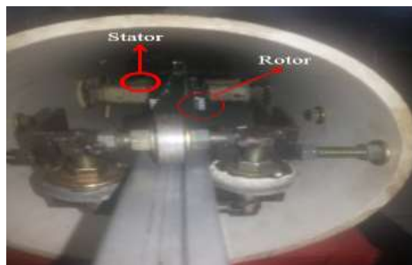
Figure 1 Construction of Generator Translation
