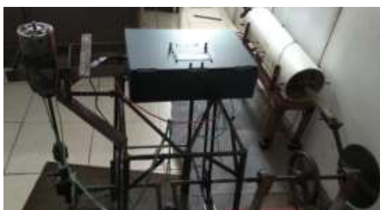
Figure 5 Schema testing of the power output for translation and rotation motion generators using Buck
