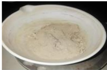
Figure 2. Zeolite synthesis after dried in an oven at 150°C for 24 hours.
