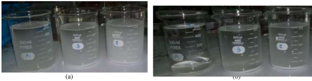
FIGURE 1. (a) Dispersion of mordenite in water at t=0 and (b) after t= 150 min.
