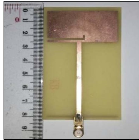
Fig 5. Fabrication of multiband antenna based on multiband slot
