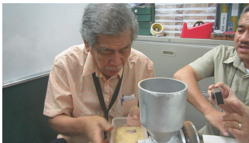
Blowing air into the ground millet to separate the hulls from the grain
