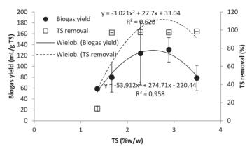
Fig. 2. Correlation between TS level on biogas yield and TS removal.
