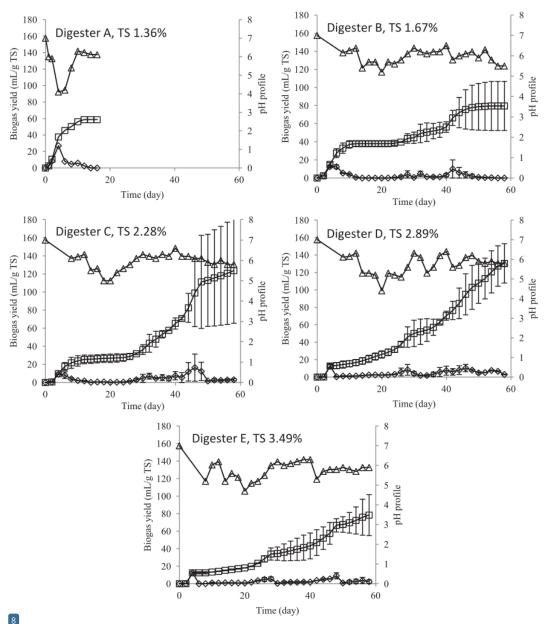
8 Fig. 1. The effect of total solid concentration on biogas production daily ( $\Diamond$ ), biogas production cumulative ( $\Box$ ), pH profile ( $\Delta$ ).
