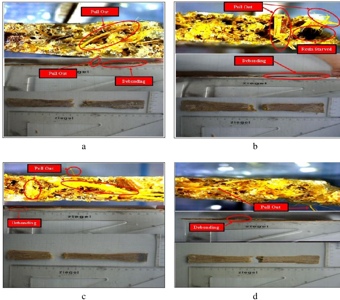
Figure 7. Macro Photo results of a composite fracture of petung bamboo fiber with polyester matrix (a) Without NaOH Soaking (b) 1 hour NaOH Soaking (c) 2 hours NaOH Soaking (d) 3 hours NaOH Soaking
